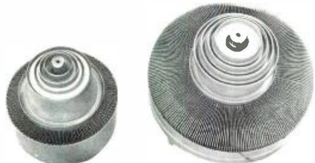
Newly designed tubes for the TTG include the aural tube (left) and the 30 kW visual tube. The cavity remains cool to the touch, according to RCA
