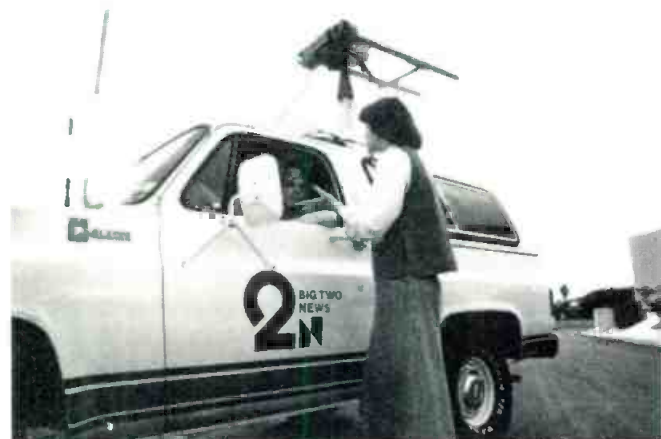
Though KPRC's Blazers are small in comparison to larger vans, they contain a potent production capacity including Microwave Associates MA-2EP 2 GHz transmitters, Nurad Dual Golden Rod antennas, Ikegami HL-77 camera, Sony BVU-50 and BVU-100 VCRs. Four-wheel drive overcomes nearly all of the common obstacles vans often find insurmountable
