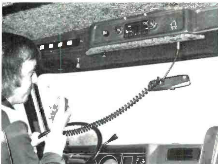
Driver of WROK van can go on the air while underway, with all equipment, including 450 MHz radio link to main studio, of top studio quality. Note sound-absorbing material to improve acoustic quality of space.
