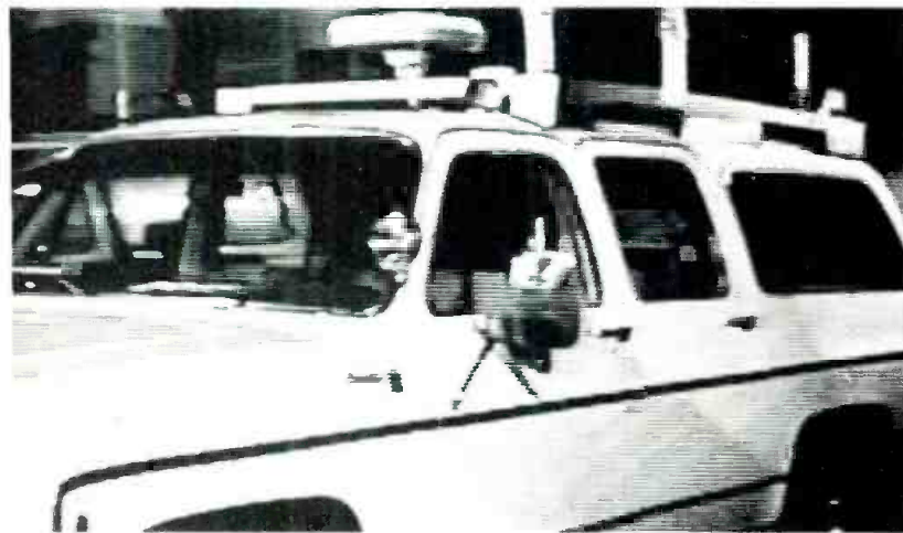
The Suburban used by WMAQ, Chicago, as its main ENG vehicle carries both 2 and 7 GHz microwave transmitters/receivers. The 2 GHz antenna is mounted forward and the 7 GHz dish is mounted aft. The routing of the signal is handled by an ENG Manufacturing-built assignment switcher (below). The switcher matches the source with the desired output and matches source and output with either frequency microwave unit
