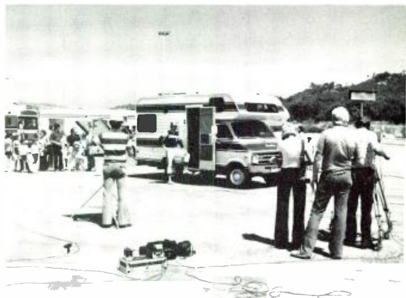
Mobile recreational vehicles are the anathema of RF mics because of their reflective surfaces. KFMB-TV solved the problem with an HME antenna diversity system. Note lighting stand-mounted antennas to right of camera and by refreshment booth.
