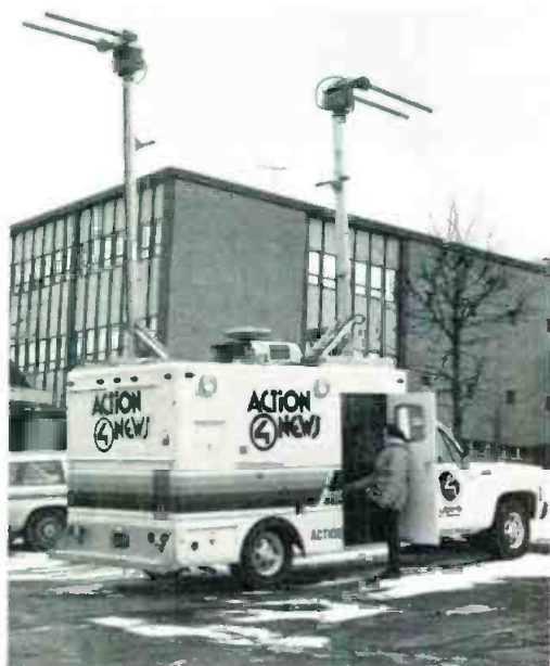
WTAE's second mobile unit is a Wolf Coach-fabricated mini-van. The units have been equipped with dual transmit/receive microwave transmitters so they can function as repeater stations for each other. Interior of the mini-van (left) represents one design philosophy in which a strong EFP production capacity is placed in the van. Other stations such as KPRC and WMAQ prefer a streamlined news-only approach
